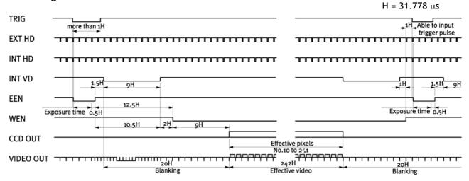
Fig. 12. Vertical timing for Edge pre-select
